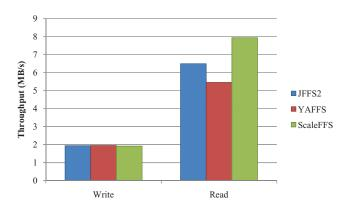
Fig. 8. The performance of read and write operations.
