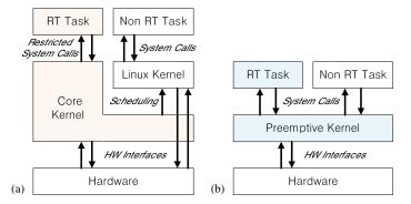
Figure 1. Kernel architectures for real-time systems: (a) sub kernel style and (b) preemptive kernel style.
