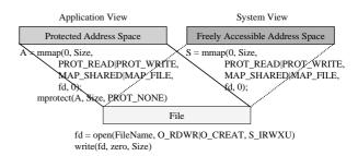
Figure 4. Mapping a file to two virtual addresses
