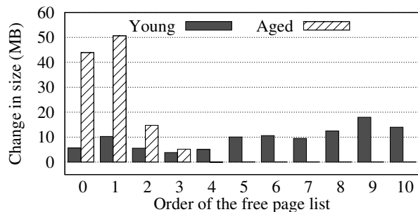
Figure 3. The change in the number of free pages in each order in the buddy allocator upon an application termination
