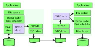
Figure 2. The structure of GNBD (GFS Network Block Device)
