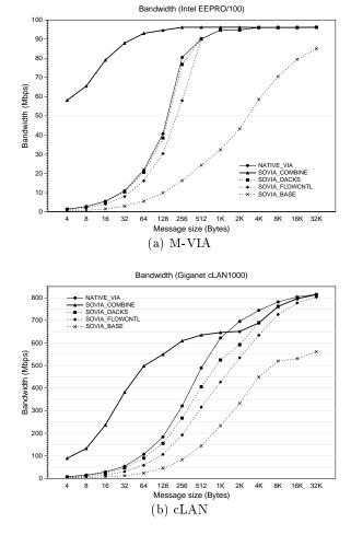
Figure 8: Impact of various optimizations on bandwidth
