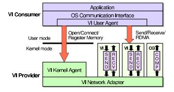
Figure 1: The organization of the Virtual Interface Architecture
