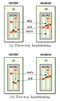
Figure 3: Synchronizing sender and receiver to satisfy the pre-posting constraint.
