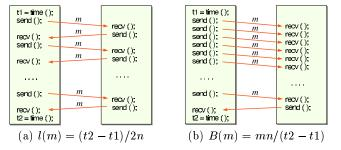
Figure 2: The structure of microbenchmarks to measure the (a) latency and (b) bandwidth. m is the packet size and n denotes the number of packets sent and received during the measurement.
