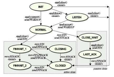
Figure 11: The state transition diagram of SOVIA
