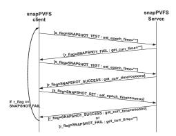
Figure 3. Message exchange between the snapPVFS server and the client
