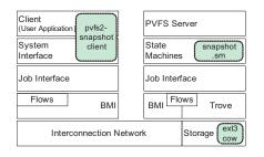
Figure 1. Structure of the snapPVFS
