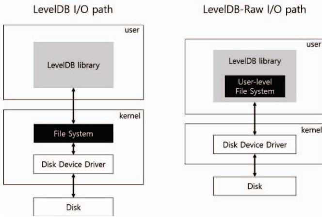
Figure 1. LevelDB &amp; LevelDB-Raw I/O path
