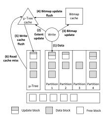
Figure 7: The overall architecture of  $\mu$ -FTL
