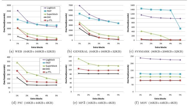
Figure 8: A performance comparison of FTLs. The values (A+B+C) in the parenthesis represent the size for per-block invalid page counter (A), the  $\mu$ -Tree cache size (B), and the bitmap cache size (C) used in  $\mu$ -FTL.
