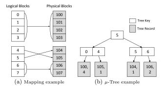
Figure 2: An example of multiple mapping granularities
