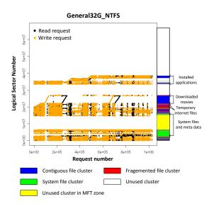
Figure 6: A disk access pattern of a general PC usage trace
