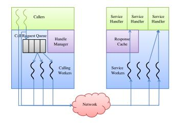
Fig. 2. FlexRPC system architecture
