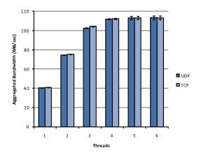
Fig. 6. Aggregated bandwidth in FlexRPC (16 KB argument size)
