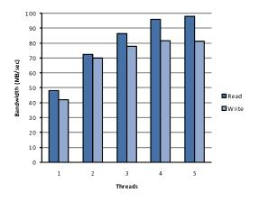
Fig. 9. Aggregated effective read and write bandwidths of Kadoop
