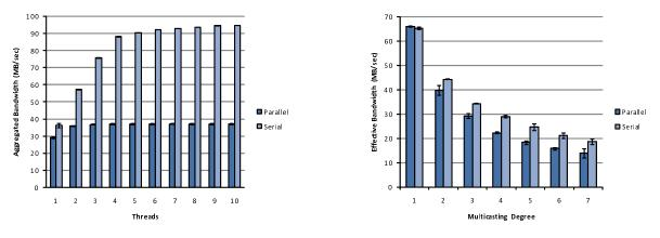
(a) Changes in the aggregated effective bandwidth (32 KB argument size with multicasting degree of three)
