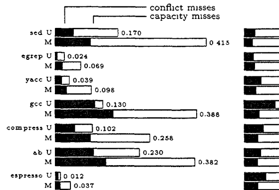
Figure 4: MCPI Caused by Cache Misses.
