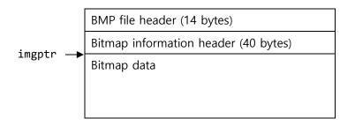
We will provide you with the skeleton codes, in which all the BMP file header and the Bitmap information header are parsed. So you don't have to worry about these headers. Before manipulating the bitmap data, we check for these headers to make sure the target image file is in the right mode, and then extract the width and the height of the image. The first argument of bmp\_mosasic(), imgptr, will point to the memory address that contains the actual bitmap data.
