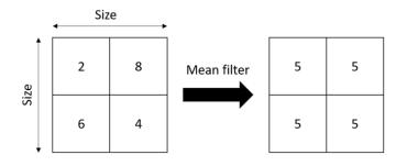
In case the image width or height is not a multiple of the given square size, we just calculate average on remaining pixels as follows.
