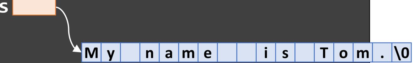
The diagram shows a variable `s` (represented by an orange box) pointing to the start of a character array. The array contains the characters 'M', 'y', ' ', 'n', 'a', 'm', 'e', ' ', ' ', 'i', 's', ' ', 'T', 'o', 'm', '.', and '\0'. Each character is enclosed in a blue box.
